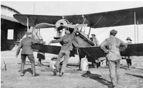
Australian ground personnel turn an S. E. 5a's propeller to start the engine
